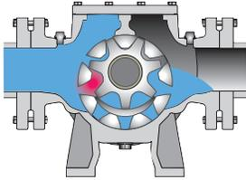
As the rotor and idler unmesh, an under-pressure is created and the liquid enters the newly created cavities.
