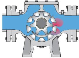
The rotor and idler mesh and liquid is pushed into the discharge line.
