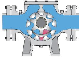
Liquid is transported in sealed pockets to the discharge side. The walls of the pump casing and the crescent create a seal, that separates suction from discharge side.
