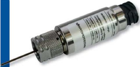
This sensor is qualified by some specific characteristics. It can be installed in any orientation and achieves highly accurate values, as it is measuring within the medium. It has IP 69 and can be installed and dismantled easily by screwing it into a 1620 series p/T-test point.
