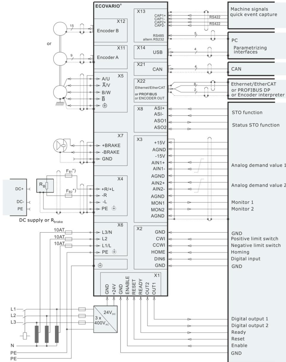
\*) not necessary if ballast resistor DPRxx is used
