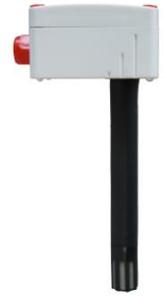
The CDI4-Series (H&T) is designed to measure relative humidity and temperature in air ducts of heating, ventilation and air-conditioning systems. The humidity sensor output is active, the temperature sensor output can be active or passive.
