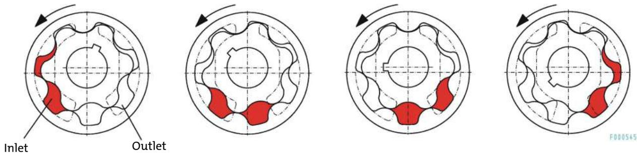
When we designed the BFP series we specifically selected the number of teeth and the width of the gerotors so the pumps have the smallest possible physical dimensions, low weight and minimal loss in efficiency. The low relative speed between the internal and external gear make the pumps extremely durable and smooth.
