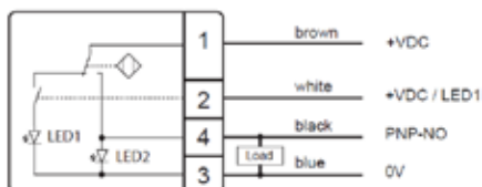
Connection diagram „P“ PNP-NO // Semi-Automatic
