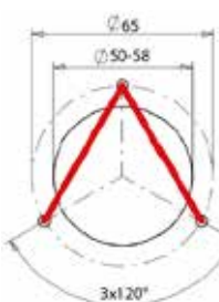
Hole pattern (A-mounting)
