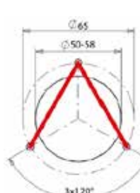
Hole pattern (A-mounting)
