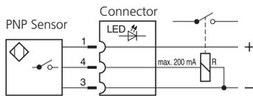
**S4** - Circuit diagram of the normally - **CLOSED** sensor
