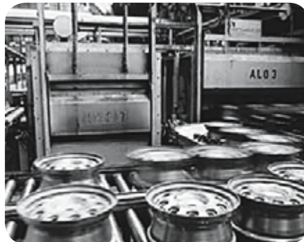
Aluminium industry: curing oven for wheel rims
