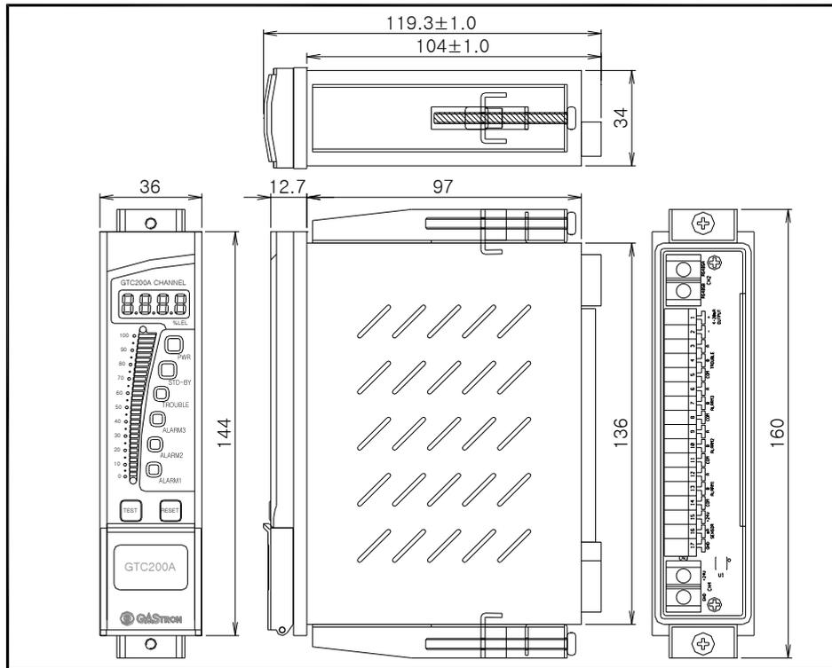
7-2. Panel Mount Type Dimension and Panel cut-out Size
