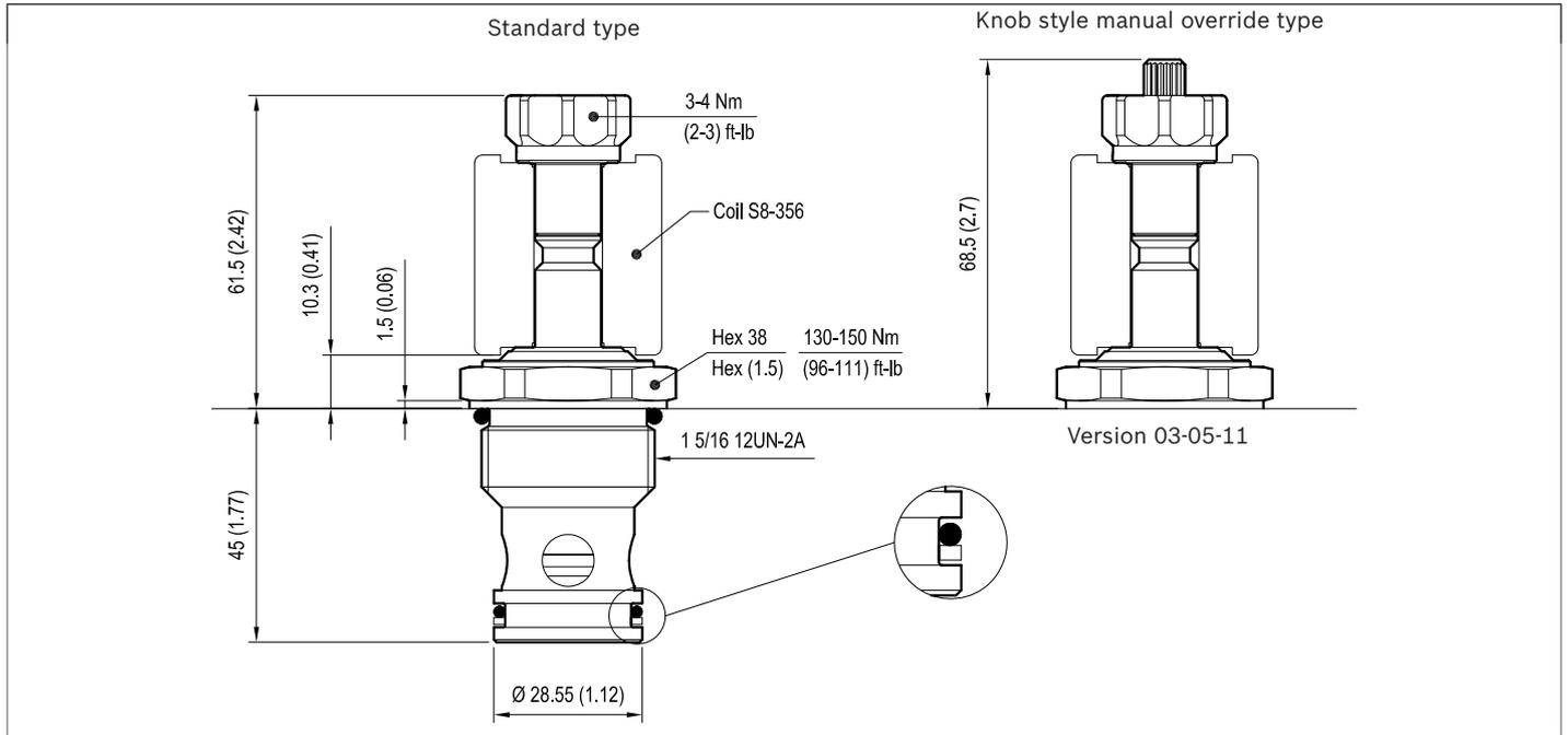
▼ **Version 03: Solenoid operated valves, poppet 2-way normally closed**
