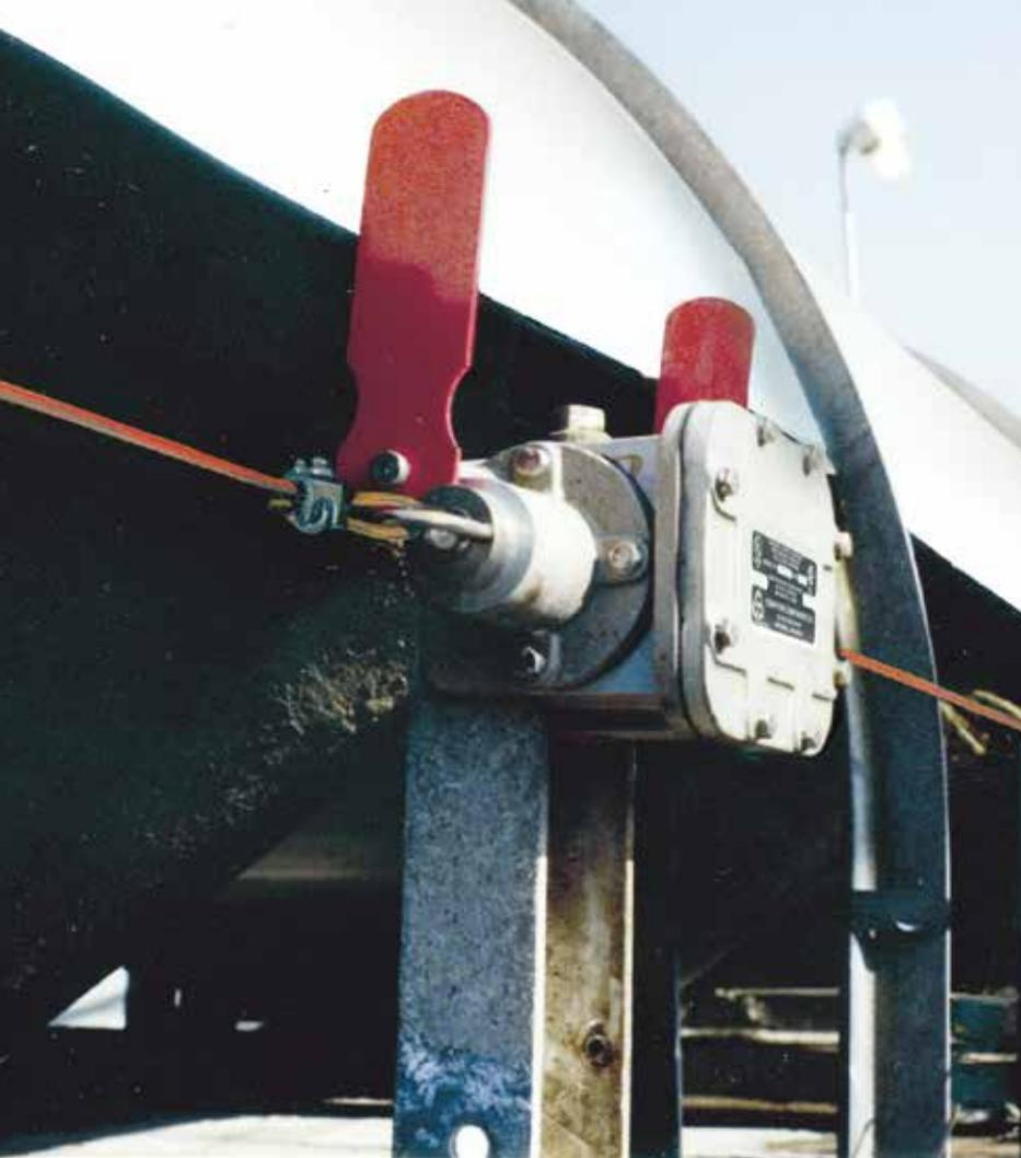
The PC Stop Control can be used for emergency shutdown of conveyor systems, elevator equipment, bulk handling systems, cranes, production and assembly lines, or any other equipment which may require immediate, positive shutdown.
