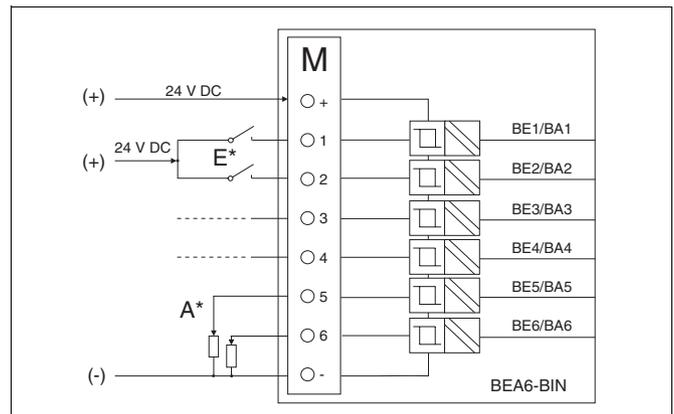
\*) Connection example: I = binary inputs; O = binary outputs
