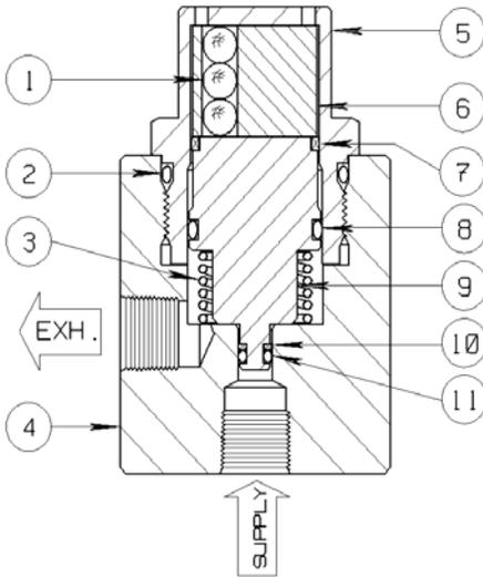
The 15RS57 Fusible Valve is a two position, two-way normally closed, **Temperature Sensitive** flow control device. Intense heat, or close proximity to a fire, will melt the solid Eutectic that maintains the valve's normally closed flow path. When the valve is subjected to heat that exceeds the actuation temperature, a Supply-to-Exhaust flow path will occur automatically.
