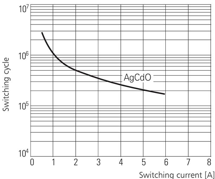
NOTE: The lifetime is dependent on the load; for heating -/ cooling operation on switching frequency.
