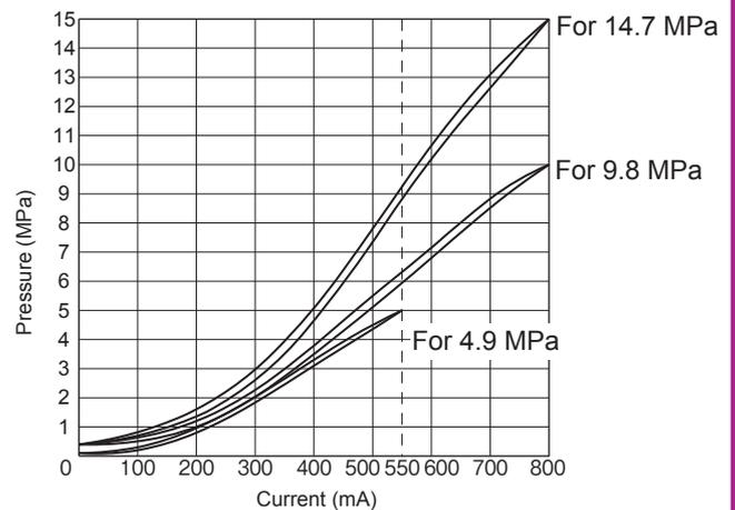
**Pressure override characteristics (viscosity 25 mm<sup>2</sup>/s (cSt))**
