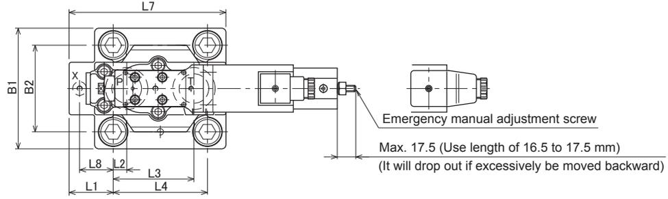
In case of electric connection symbol B (DIN connector GDM3011)
