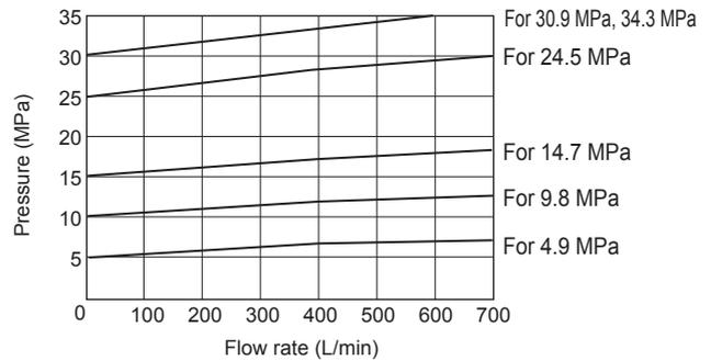
**Minimum adjustment pressure characteristics (viscosity 25 mm<sup>2</sup>/s (cSt)) Input current: 0**
