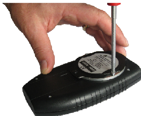
Figure 31: Removing the grid (part 1)
