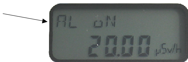
Figure 2: MiniTRACE CSDF display – alarm is activated
