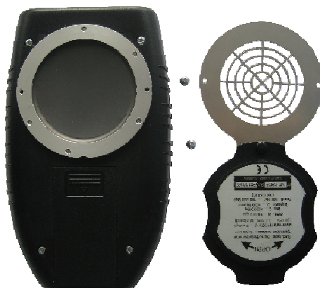
Figure 32: Removing the grid (part 2)
